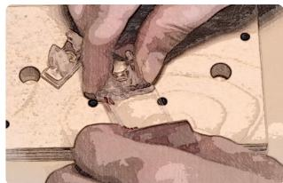
**D.** Align and firmly press false front against false front clips. Remove false front by pulling straight off cabinet, (clips should remain on front). Secure clips to false front using #6x5/8" screw supplied.
