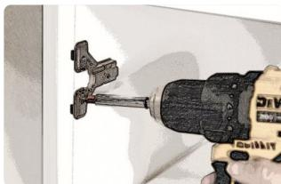
**G.** Clip top hinge to top hinge plate. When door is properly positioned, screw lower hinge plate into place. Apply rubber bumpers to corners of doors, opposite of hinges.
