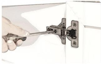
**I.** Final, **VERY IMPORTANT** step. Find bag labeled "Screws for Back Hole of Frameless Hinge Plates". Screws are required for long-term strength of hinges. Without these, doors may come loose over time. Insert one at back of plate.
